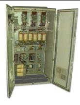
frequency converter 3-phase 15kVA input 3x400V 50/60Hz, output 3x 115/200V 400Hz, Y connection 5kVA per phase, 8,5kVA (25kVA) for 2-3 minutes, instruments and potentiometer for voltage. Cabinet L 800 H 1800 T 600 mm IP20
